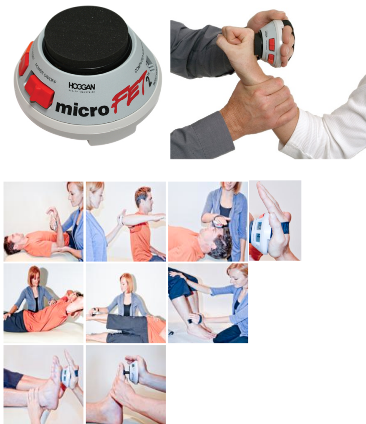
Figure A.2. Hand-held force sensor microFET2 and its neuromuscular-musculoskeletal usage in force evaluation and testing (FET). Selectable units of measure can be pounds (lbs.), Newtons (N), kilogram-force (kgf). The threshold is variable and settable from .8 lb to 300 lbs. Information from the gauge is displayed in two LCD windows, peak forces and duration/sec.
