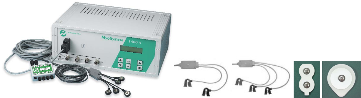
Figure A.10. Myosystem 1400A with standard 2/3-pin leads and dual/single electrodes, and the connection box was built to connect Myosystem 25-pin D-sub port to Optotrak ODAU BNC .
