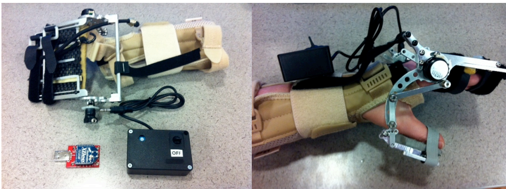
Figure 2.11. The image on the left shows the independent parts of the system including the red XBEE explorer that plugs into the USB port of the computer. The image on the right shows the system on a person.
