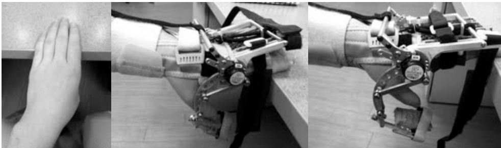
Figure 2.10 A. Shows what the hand is doing without the device on. B and C show the process with the HandSOME device on.
