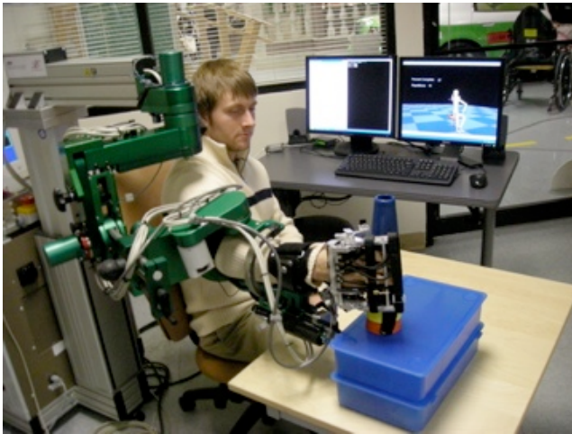
Figure 3.5 ARMin III robot and passive hand device, HandSOME, being used in functional shelf task in time-independent functional training mode.
