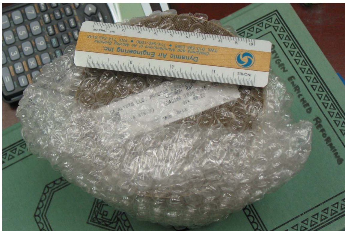
Figure 3.7 BASF catalysts ATR-7B prior to coring. Washcoated cordierite dimensions of 127 mm diameter and 101.6 mm depth.
