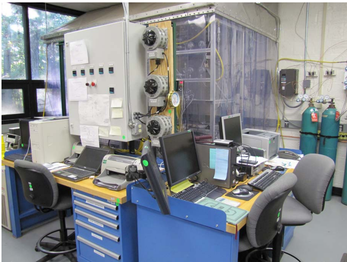
Figure 3.17 Laboratory reformer test apparatus, control and work space. Desk with multiple computer LCD monitors is the operator control desk. Large gray panel on the left is the electrical power and signal distribution panel. Walk-in hood is shown in the background of the photo.
