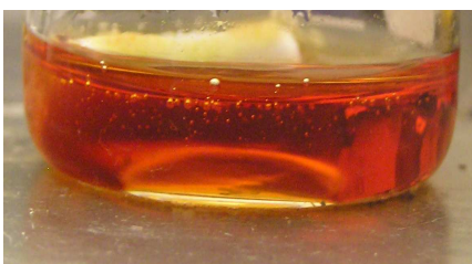
Figure 6.1 PVA beads were dissolved in FeGa aqueous solution
