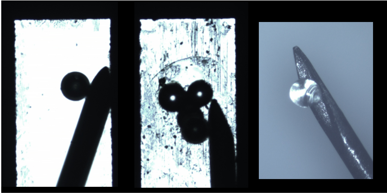
Figure 5.16: Manipulation of spheres using wetted needle. Left and center: Placement of glass spheres on cantilever. Right: Glass sphere held on needle bevel with water.
