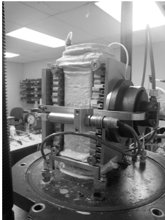
Figure 5.2.3. Picture of True Triaxial Horizontal Loading System with Horizontal LVDTs.
