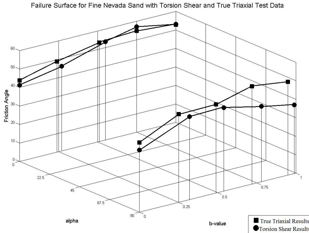
Figure 7.1.12. Comparison of 3D failure surface plot for True Triaxial and Torsion Shear tests.
