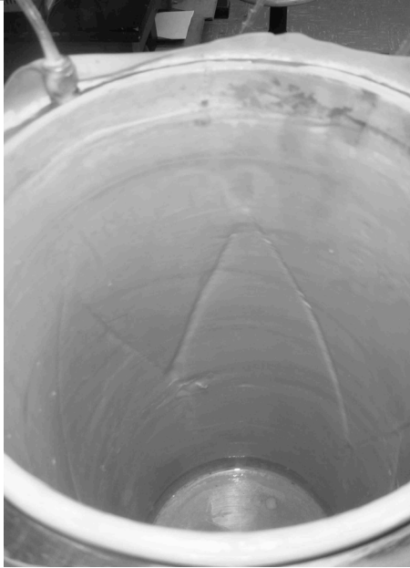
(a) Outside & Inside Shear Bands (Test 2; ( \alpha=0^\circ , b=0.75 ))
