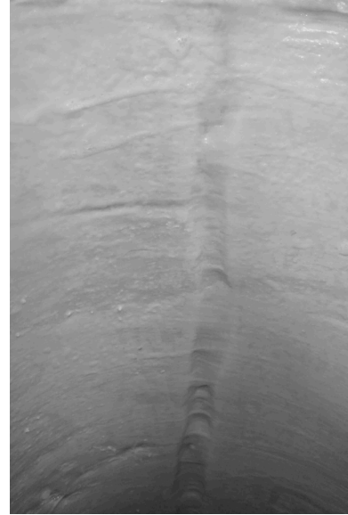
(b) Outside & Inside Shear Bands (Test 26; ( \alpha=0^\circ , b=1 ))
