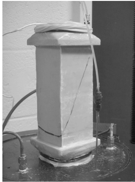
Figure 9.2.1. Typical example of shear band development for most True Triaxial tests.
