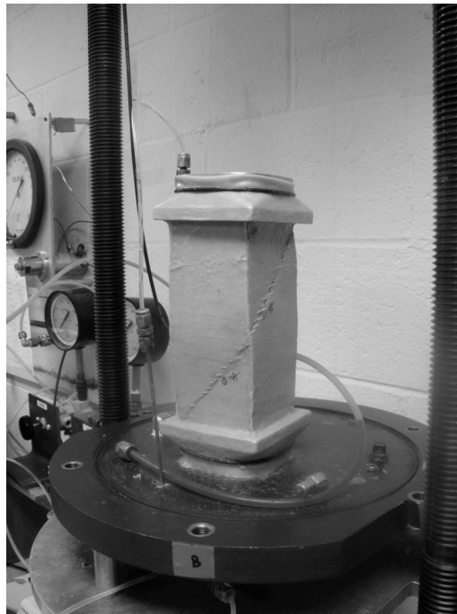
Figure 9.1.1. Example of sheared specimen with two distinct shear band planes after failure in triaxial testing.
