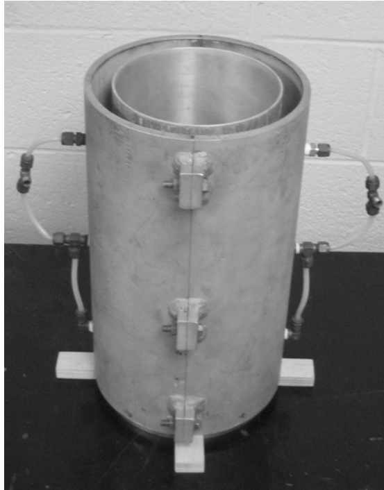
Figure 4.12: Mold for the hollow cylinder torsion shear tests.
